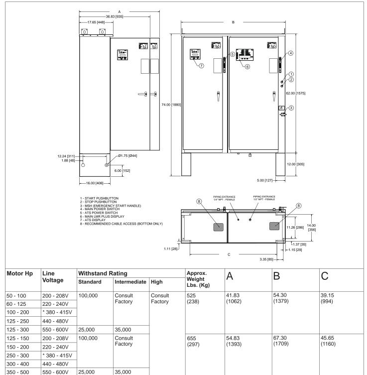
\* Coils Available: 380V-50Hz, 380V-60Hz, 415V-50Hz, 415V-60Hz
